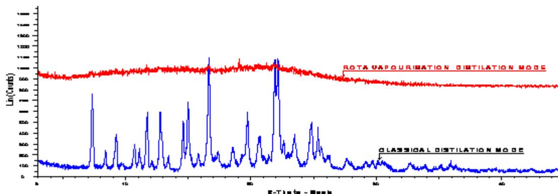
Figure 5. pXRD of Crude 1 obtained from Rota vapor and classical mode of distillation process
