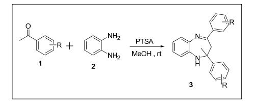
**Reagents and Reaction conditions-** *o*-phenylenediamine (1equiv.), different acetophenone (2.5 equiv.), MeOH, rt, 2-5 hr
