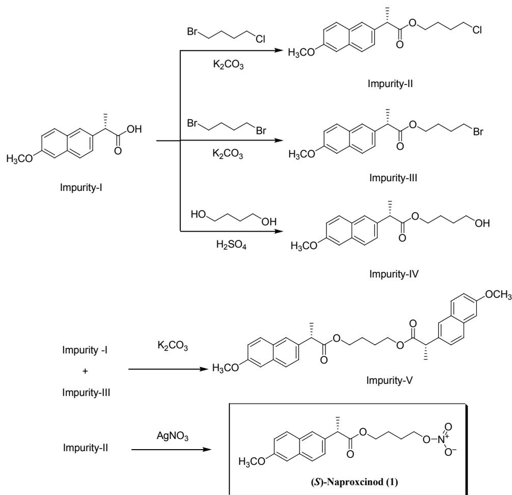
**Scheme 1: Synthesis of Naproxinod and its Impurities (II, III, IV and V)**
